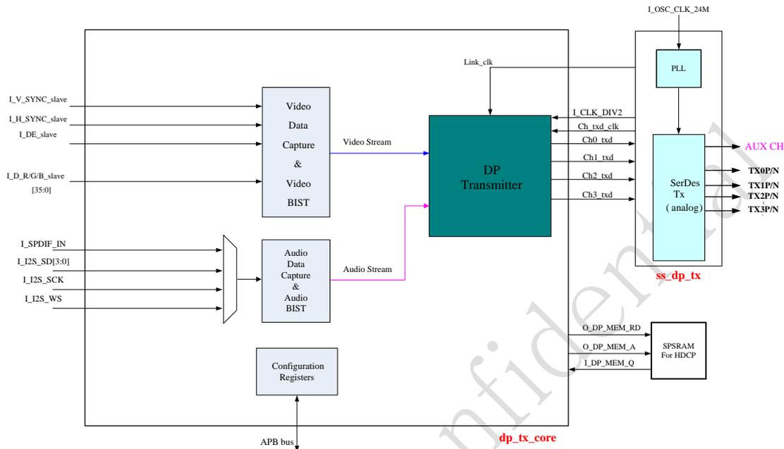
Fig. 34-1 eDP TX controller Block Diagram
