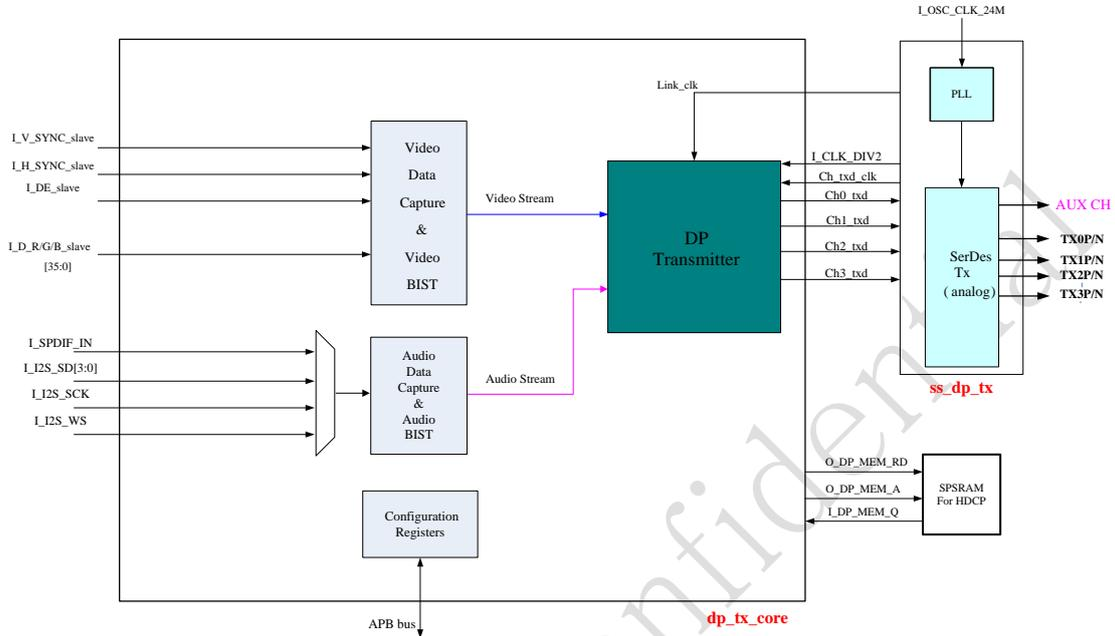
Fig. 34-1 eDP TX controller Block Diagram
