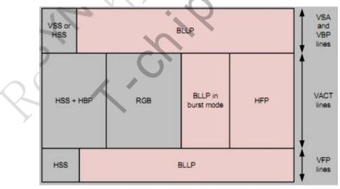
Fig. 37-7 Command Transmission Periods within the Image Area
