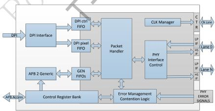
Fig. 37-1 MIPI Controller architecture
