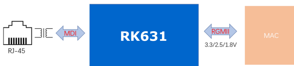
Fig. 3-1 UTP<->RGMII Application Transmit Functions
